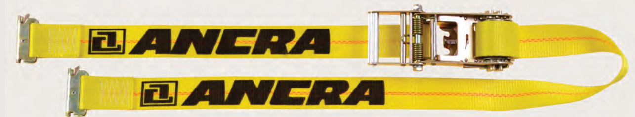
Series E Heavy-Duty Buckle Strap w/ Spring E Fitting Heavy-duty 12,000 lbs. yellow latex treated polyester webbing. WLL: 1,333 lbs./605 kg. Fixed End: 48-in.
