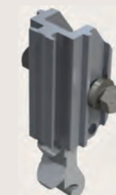
50187-31 Lift-A-Deck II Low Profile Foot Assembly. Machined guide shoe allows for inspection of both locking lugs while beam remains installed in the track. Features a coil spring for optimum service life. Weight: 0.6 lbs./27 kg.
