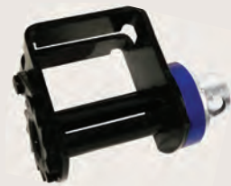
49207-137-RW Standard Ratchet Winch Double L Track Slider Lighter 7mm heat treated frame Weight: 8.0 lbs./3.6 kg. WLL: 5,500 lbs./2,500 kg.
