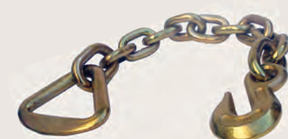
43366-14 Chain Anchor with Delta Ring for 3" & 4" Strap Assemblies. 3/8", G43 Chain and 3/8" G70 Grab Hook, gold zinc plated. WLL: 5,400 lbs./2,450 kg. Weight: 3.4 lbs./1.54 kg.
