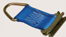
40386-10 Series E and A Rope Tie Off 3-piece end fitting for use with Series E or A Track. WLL: 1,000 lbs./454 kg. Weight: .30 lb./0.14 kg.
