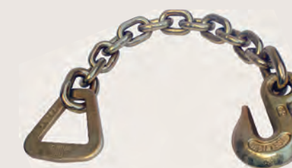
43366-21 Chain Anchor with Delta Ring for 2" Strap Assemblies. 5/16", G43 Chain and Grab Hook, gold zinc plated. WLL: 3,330 lbs./1,510 kg. Weight: 2.55 lbs./1.16 kg.
