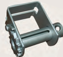
49207-127-XZ Web Storable Double L Track Slider X-Treme Zinc Finish Lighter 7mm heat treated frame Weight: 6.8 lbs./3.1 kg. WLL: 5,500 lbs./2,500 kg.
