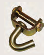
49914-11 Low Profile Swivel J Idler Hook Heat treated w/ gold zinc finish. WLL: 3,333 lbs./1,515 kg. Weight: .87 lb./40 kg.
