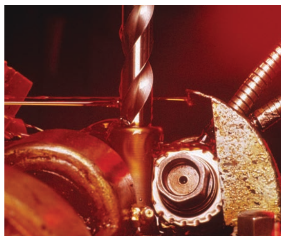
Flute milling of large diameter twist drills
