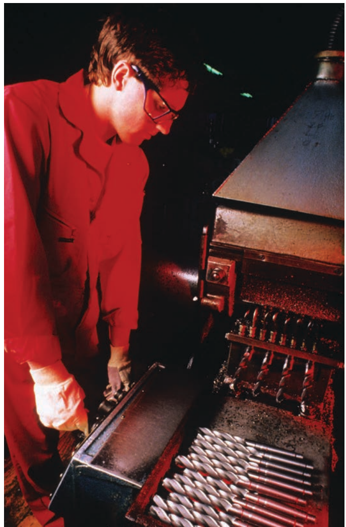
Flute milling of taper shank drills
