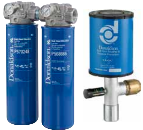
X011449 Clean & Dry Kit includes single head (2), high efficiency diesel filter, water absorbing filter, pressure gauge (2) and T.R.A.P.™ breather. For flow rates up to 50 GPM / 189 LPM
