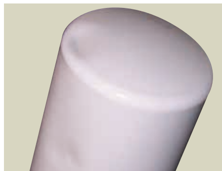
Dents in a steel filter canister create a concentration of stress, making the canister more susceptible to fatigue.
