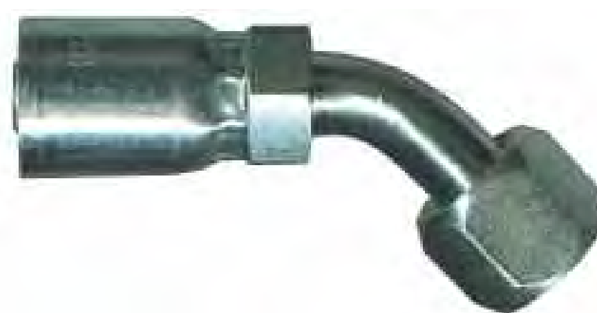
45° ELBOW S.A.E. 37° Female Flare (Swivel)
