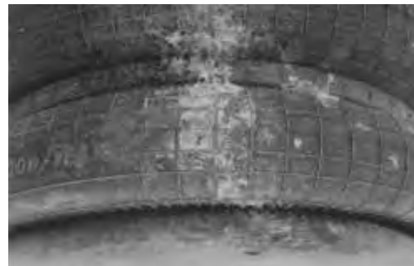
DAMAGE FROM CHEMICALS
