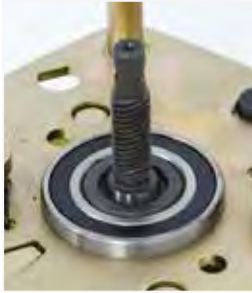
Maintenance free sealed bearings reduce operator effort
