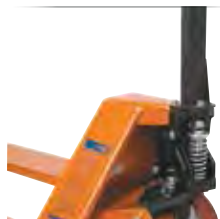
Totally sealed H.D. hydraulic unit steel wheel wrapped in polyurethane
