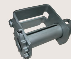
49207-187-XZ Low Profile Double L Track Slider X-Treme Zinc Finish Lighter 7mm heat treated frame Weight: 6.2 lbs./2.8 kg. WLL: 5,500 lbs./2,500 kg.
