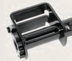
49207-187 Low Profile Double L Track Slider Lighter 7mm heat treated frame Weight: 6.2 lbs./2.8 kg. WLL: 5,500 lbs./2,500 kg.
